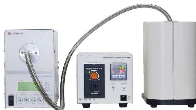
UV light source* (UV-1047Xe with Xe lamp)
